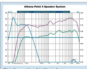
HT Labs Measures: Athena Point 5 Speaker System This graph shows the quasi-anechoic (employing close-miking of all woofers) frequency response of the S.5 satellite (purple trace), P.5 subwoofer (blue trace), and C.5 center channel (green trace). All passive loudspeakers were measured at a distance of 1 meter with a 2.83-volt input and scaled for display purposes.
