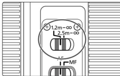
You can set the focusing distance range to 1.2 m/3.9 ft. to infinity or 2.5 m/8.2 ft. to infinity. By setting the suitable focusing distance range, the actual autofocus time can be shorter.
