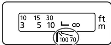
The infrared index corrects the focus setting when using monochrome infrared film. Focus on the subject manually, then adjust the distance setting by moving the focusing ring to the corresponding infrared index mark.
