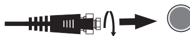
Satellite, cable or TV antenna cable to TV ANTENNA terminal (cable not included)
