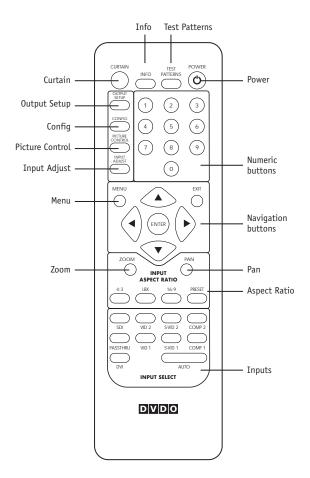
The iScan HD Infrared Remote Control (IRC) offers more functionality and convenience than the front panel control buttons. Unlike the front panel controls, the remote control has a complete set of navigation buttons: Left, Right, Up, Down, Enter, and Exit. The remote control buttons have slightly different behavior than the corresponding front panel buttons. The remote control buttons and their control actions are described below.
