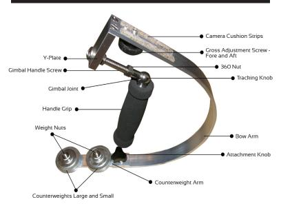
Gimbal Joint and Handle Grip: The design of the Glidegear 3000 is engineered to stabilize the camera by moving the center of gravity below the camera and under the actual gimbal joint. The gimbal will not permit any angular disturbance to pass through it, so the shakes and bumps caused by your hand or anything attached to your hand will be absorbed by the gimbal and isolated from the camera.
