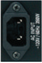
Figure 34 – AC Power Input
