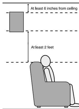
speakers should be located so that the bottom of the cabinet is at least two feet higher than the listeners' ears when the listeners are seated in the desired area.
