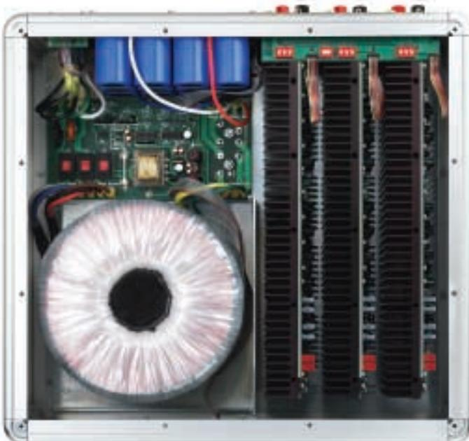
As with the Theater Amplifier Standard, the gain stages use Krell Current Mode™, discrete Class A, fully complementary circuitry. The driver/output stages employ 14 high-current transistors per channel for high output current capability. This design delivers the clean, powerful, detailed reproduction that is the hallmark of Krell amplifiers.
