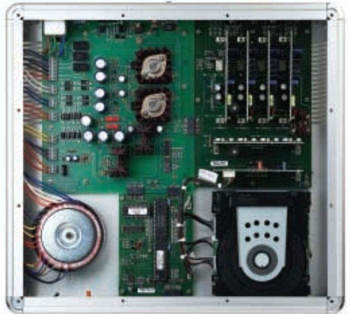
Two 24-bit ultra-high-resolution digital-to-analog converters per channel provide fully balanced operation with exceptional reproduction quality. The analog stage features Krell Current Mode™ discrete Class A, direct-coupled, fully complementary circuitry.
