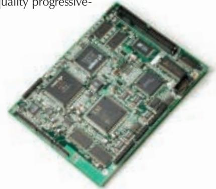
Video output is optimized for the latest solid-state video display technologies, including plasma, LCD, DLP, and DILA. The progressive-scan output employs triple 10-bit DACs and provides both RGB and component interfaces.
