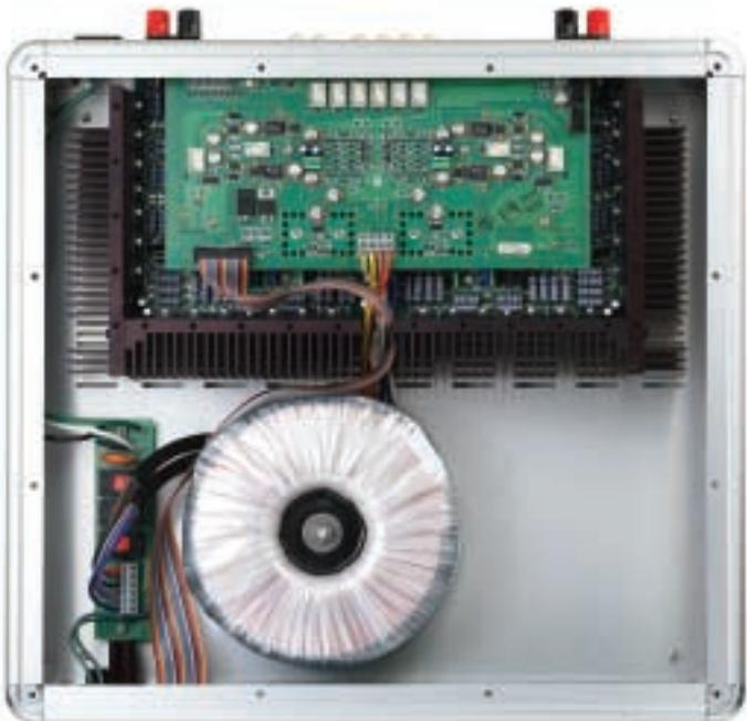
The power amplifier section incorporates proprietary Krell driver and output transistors. 12 devices per channel provide enormous output current capability—far beyond that of typical integrated amplifiers.
