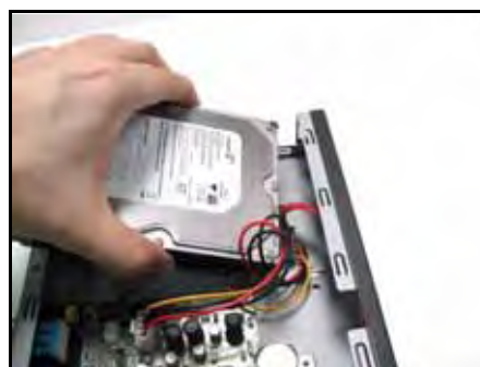
Figure 27.5 Insert the drive carefully
