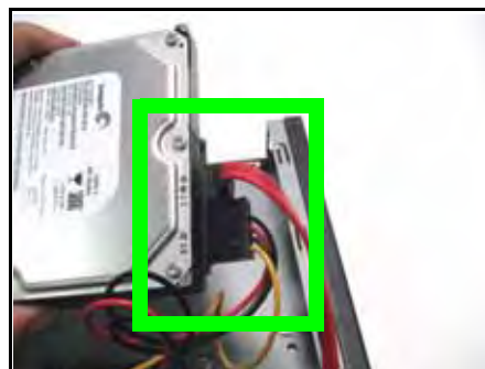
Figure 27.4 Connect the power and data cables.
