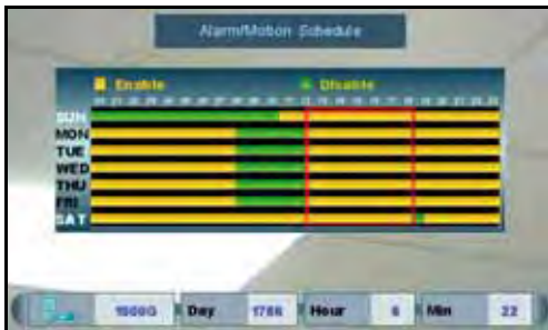
Figure 13.5 Alarm/Motion Schedule (8/16-channel only )
