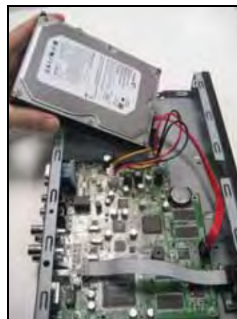
Figure 27.3 Carefully remove the HDD from housing.
