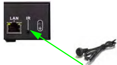
Figure 1.3 Connect the Flex IR extender
