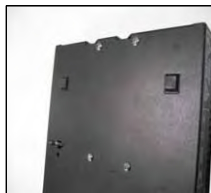
Figure 27.6 Replace the mounting screws
