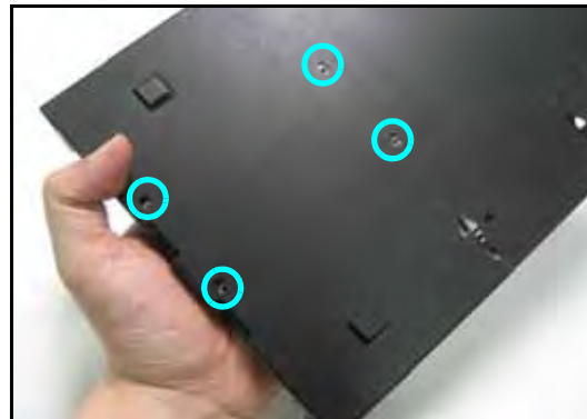
Figure 27.2 Support the HDD with your hand and remove mounting screws.
