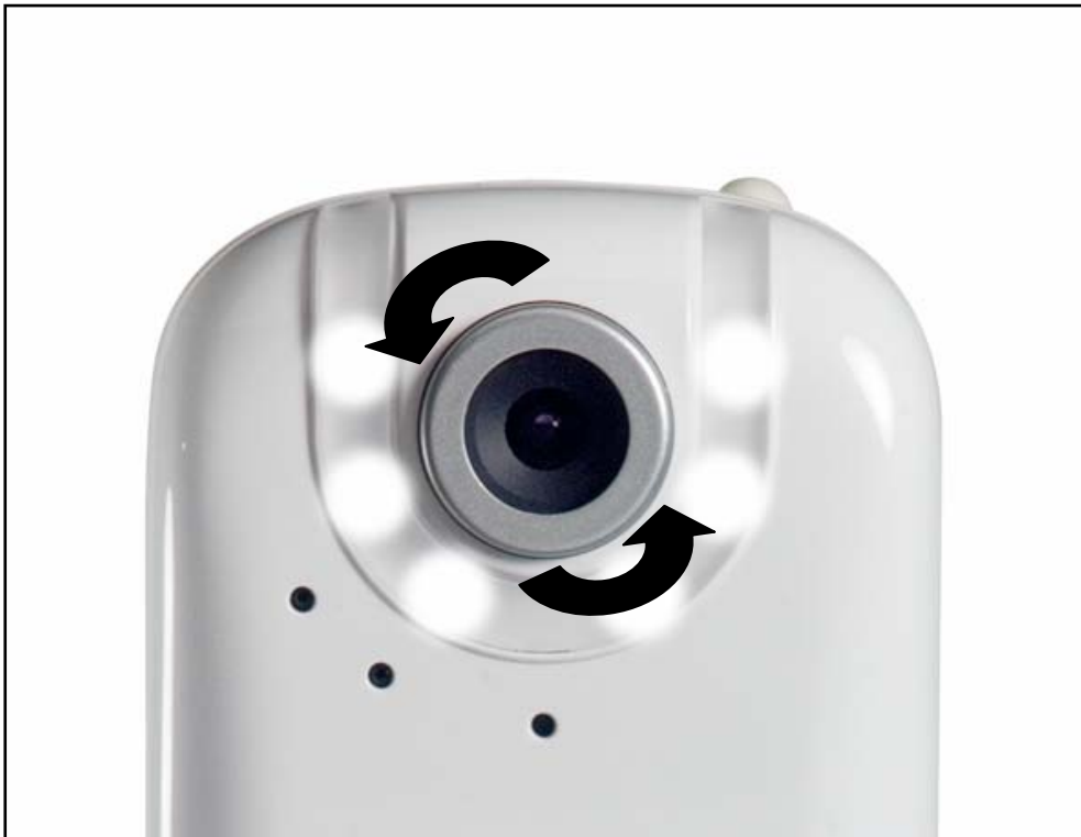
Figure 8.0 Turn the ring back and forth to adjust the focus
