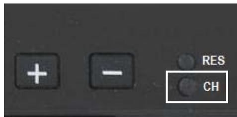
Figure 9.0 Press and hold the RES and CH buttons at the same time
