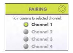
**NOTE:** If you pair a new camera to a channel which is already being used by an existing camera, the new camera will be connected to that channel. The old camera will automatically be disconnected.
