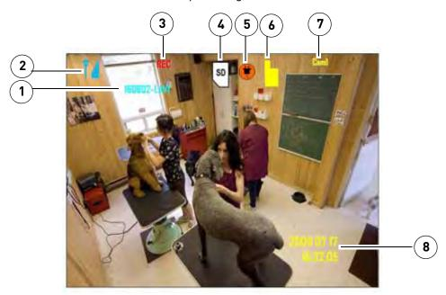
1 **File Name:** The name of the file actively being recorded. This file will appear in the file list on the SD card. The Recording File stamp indicates the hour, minutes, and seconds that the system started recording.
