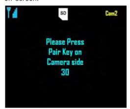
NOTE: If you do press the Pair button on the camera during the 30 second pairing window, repeat steps 2~5 to try the pairing process again.
