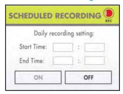
Use Schedule Recording to have the system automatically record continuously from a selected camera, or from Auto Sequence Viewing Mode according to a start and stop time.
