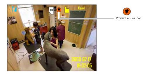
**NOTE:** The flashing icon appears only if the system was actively recording when the power failure occurred. The flashing icon will disappear when you press buttons on the receiver or remote control.
