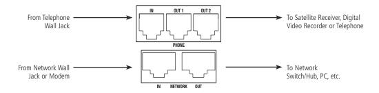
**NOTES:** The HDP 1400G is not intended for hook-up of any phone which carries two separate phone lines on a 4-pin RJ11 jack.
