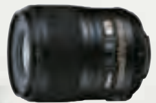
AF-S Micro NIKKOR 60mm f/2.8G ED Features Nano Crystal Coat, an ED glass element, three aspherical lens elements for the first time in a micro lens, a fast-and-quiet silent wave motor, a closest shooting distance of 0.6 ft., and a reproduction ratio of up to 1:1
