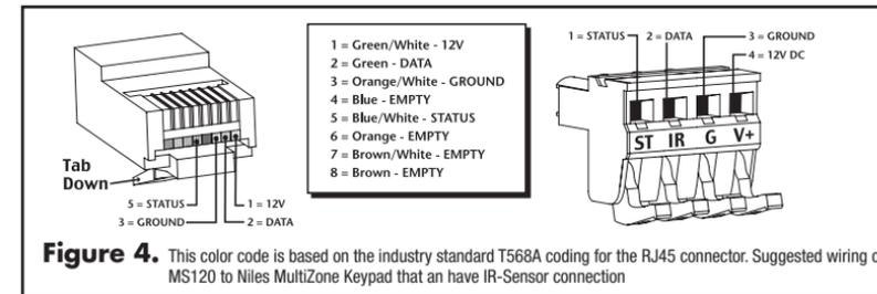
**Figure 4.** This color code is based on the industry standard T568A coding for the RJ45 connector. Suggested wiring of MS120 to Niles MultiZone Keypad that have IR-Sensor connection
