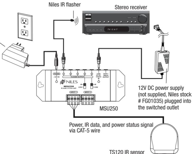
**Figure 2** Connecting the TS120 to a Niles MSU250 IR main system unit broadcasting a status feedback signal.
