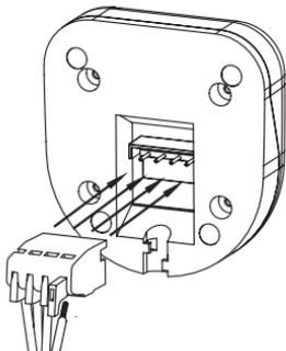
**Figure 5** Installing the removable connector
