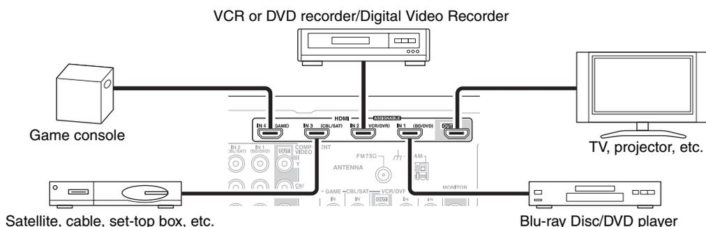
Connect your components to the appropriate jacks. The default input assignments are shown below.
