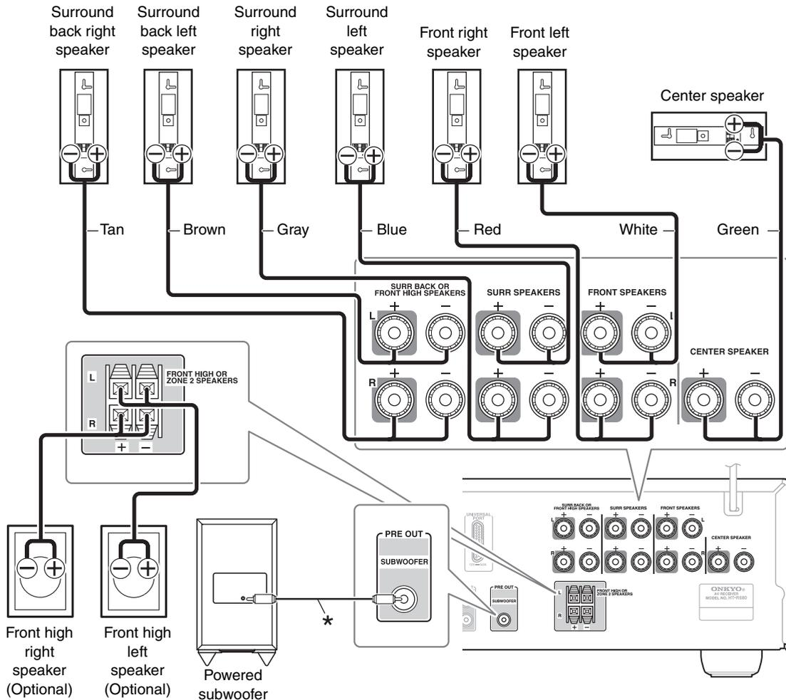
\* Using the supplied RCA cable, connect the subwoofer's **LINE INPUT** jack to your AV receiver's **SUBWOOFER PRE OUT** jack.
