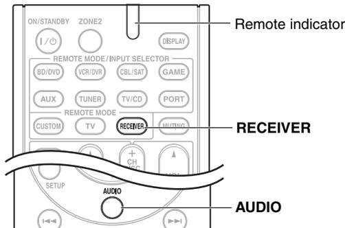
To reset the remote controller to its factory defaults, while holding down **RECEIVER**, press and hold down **AUDIO** until the remote indicator lights (about 3 seconds). Within 30 seconds, press **RECEIVER** again.
