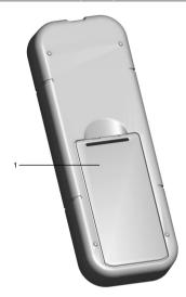
1. Battery compartment: Uses 2 x UM-4 (AAA) 1.5V
