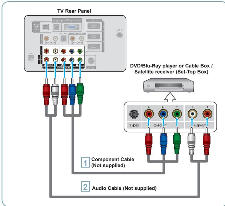
**1** Connect a Component Cable between the COMPONENT IN (1 or 2) [Y, Pb, Pr] jacks on the TV and the COMPONENT [Y, Pb, Pr] jacks on the DVD/Blu-Ray player or Cable Box/Satellite receiver (Set-Top Box).
