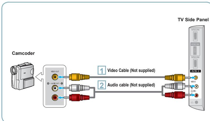
**1** Connect a Video Cable between the AV IN 2 [VIDEO] jack on the TV and the VIDEO OUT jack on the camcorder.
