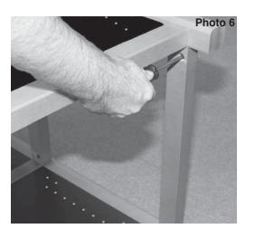
**Step 13:** Use a philips screwdriver to install (4) Shelf Pins (g) behind each lower Stretcher. Place Shelves without wood band into the cabinet behind the lower Stretchers. For orientation, pre-installed plastic pieces that lock shelves into place are closer to the <u>back</u> of the shelf. (Photo 8) Shelves lock down into place with a light tap.\*\* See Note at the bottom of this page.
