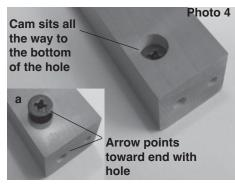
**Step 4:** Press (2) Cams (a) into each stretcher and each Back Rail. Make sure the arrow on the Cam lines up with the hole on the end of each stretcher and each Back Rail. Also be sure the Cams are pressed all the way to the bottom of each hole. (Photo 4)
