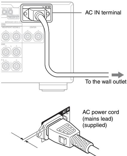
A several space is left between the plug and the rear panel even when the power cord (mains lead) is inserted firmly. The cord is supposed be connected this way. This is not malfunction.
