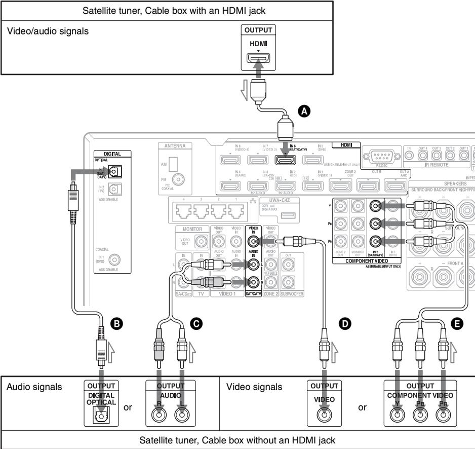
It is not necessary to connect all the cords. Connect cords according to the jacks of your equipment.
