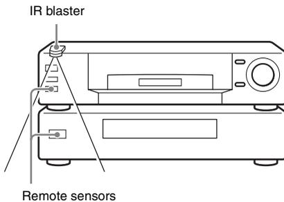
If the remote sensors on more than one device do not line up as shown in the illustration above, use another IR blaster (supplied) and another IR REMOTE OUT jack.
