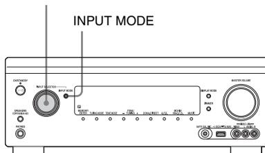
**1** Select the input source using **INPUT SELECTOR** on the receiver.
