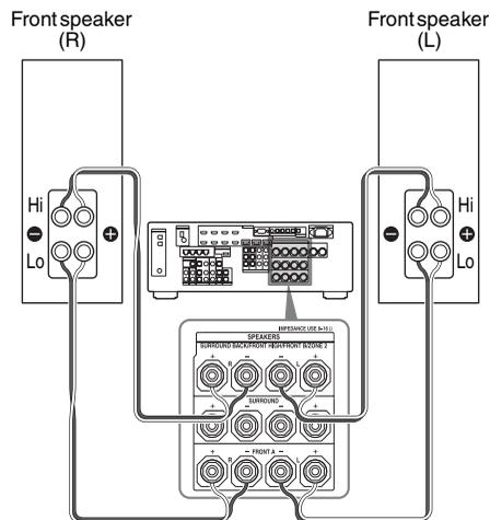
Connect the jacks on the Lo (or Hi) side of the front speakers to the FRONT A terminals, and connect the jacks on the Hi (or Lo) side of the front speakers to the SURROUND BACK/FRONT HIGH/FRONT B/ZONE 2 terminals. Make sure that metal fittings of Hi/Lo attached to the speakers have been removed from the speakers to avoid receiver malfunction.
