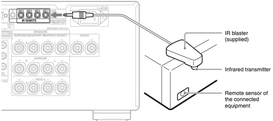
Place the equipment and the IR blaster as follows when you want to operate more than one device with the IR blaster.
