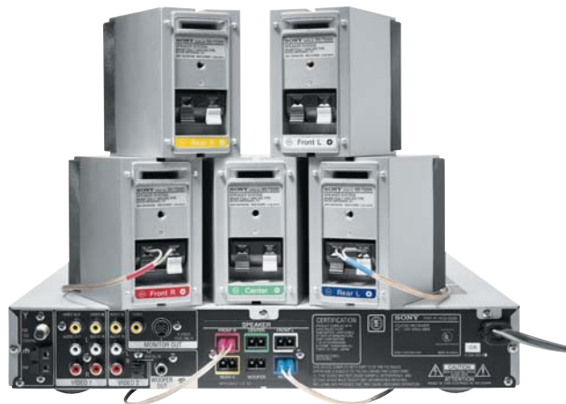
The rear of a Sony DVD Dream System, showing color-coded cables and color-coded speaker terminals.
