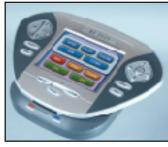
When not in use, the MX-3000 sits on its recharging cradle, which indicates a full charge with a blue LED.
