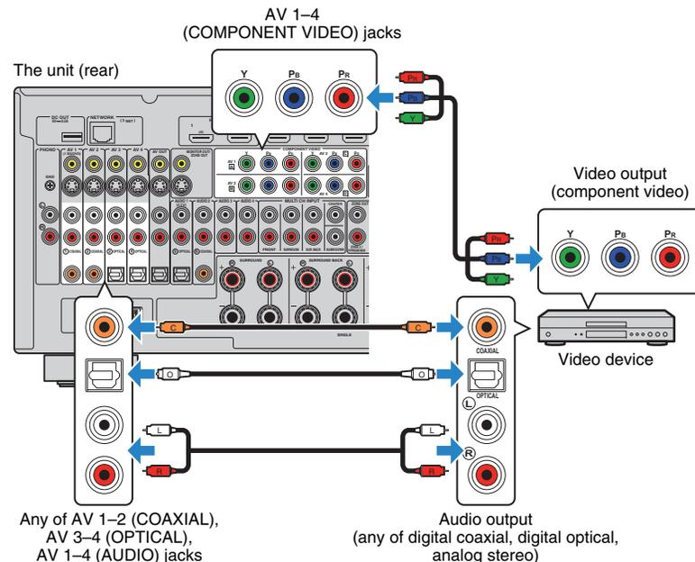
If you select the input source by pressing AV 1-4 on the remote control, the video/audio played back on the video device will be output from the unit.
