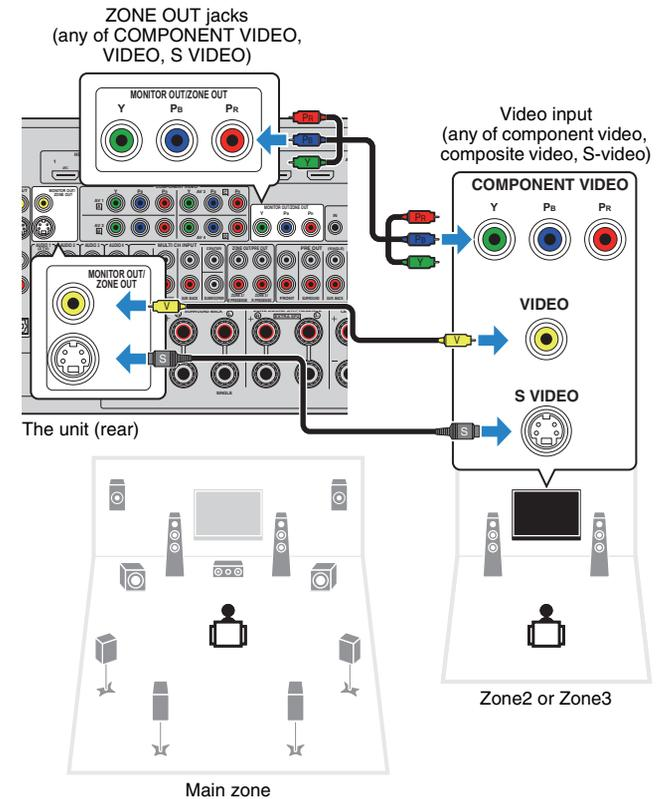
To assign the MONITOR OUT/ZONE OUT jacks to the video monitor for Zone2 or Zone3, set "Monitor Out Assign" (p.128) in the "Setup" menu to "Zone2" or "Zone3".
