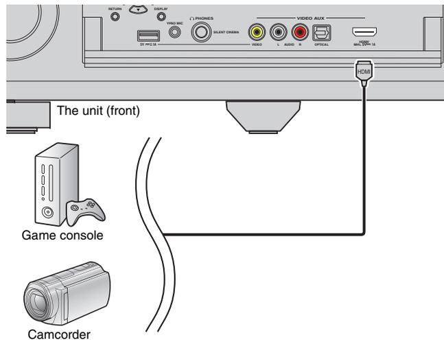
If you select “V-AUX” as the input source by pressing V-AUX on the remote control, the video/audio played back on the device will be output from the unit.
