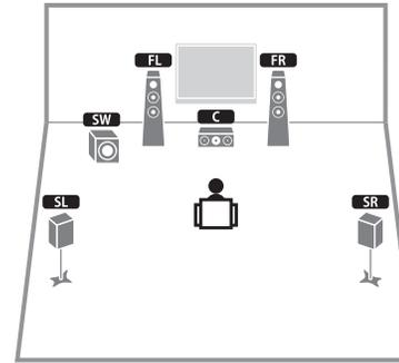
This speaker system creates front Virtual Presence Speaker (VPS) using the front, center and surround speakers to produce a 3-dimensional sound field, and is suited for enjoying 5.1-channel contents.
