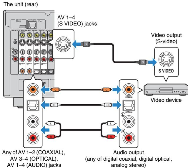
If you select the input source by pressing AV 1-4 on the remote control, the video/audio played back on the video device will be output from the unit.
