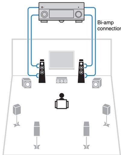
**Combining with an external power amplifier (Hi-Fi amplifier, etc.) to build an extended system**
