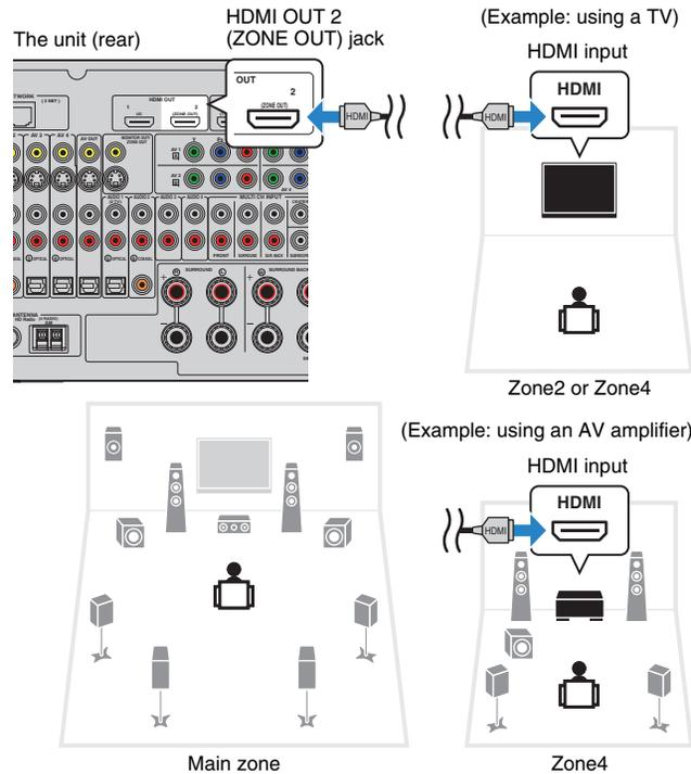
To assign the HDMI OUT 2 (ZONE OUT) jack to Zone2 or Zone4, set "HDMI OUT2 Assign" (p.129) in the "Setup" menu to "Zone2" or "Zone4".
