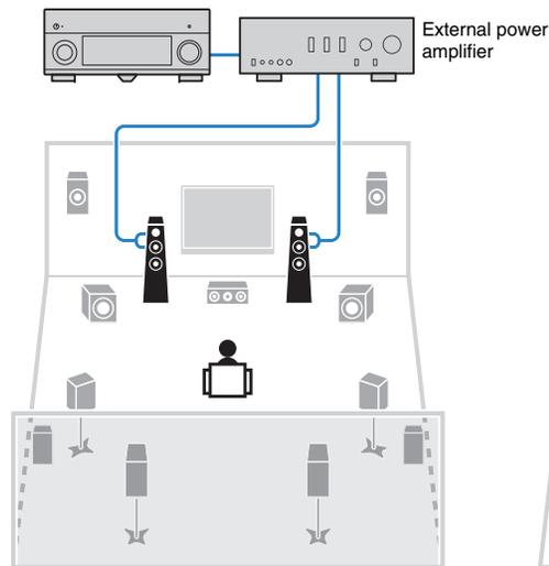
**Using the excess internal amplifiers for stereo speakers in another room**
