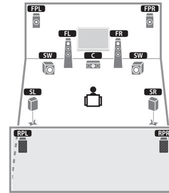
This speaker system uses the front and rear presence speakers to produce a highly-natural 3-dimensional sound field, and is suited for enjoying 5.1-channel contents.
