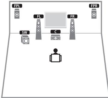
This speaker system uses the front presence speakers to produce a natural 3-dimensional sound field, and creates the virtual surround speakers using the front speakers to allow you to enjoy multi-channel surround sound (Virtual CINEMA DSP).
