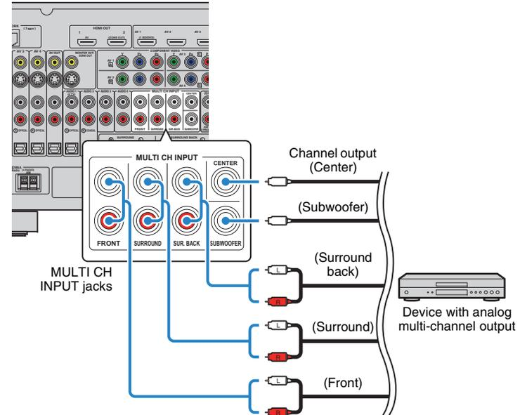
If you select "MULTI CH" as the input source by pressing MULTI on the remote control, the audio played back on the device will be output from the unit.
