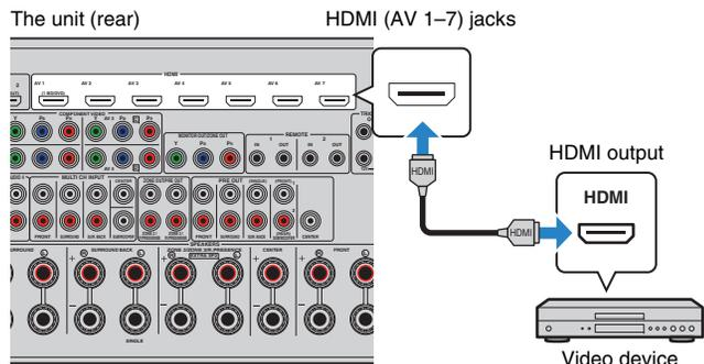
If you select the input source by pressing AV 1-7 on the remote control, the video/audio played back on the video device will be output from the unit.
