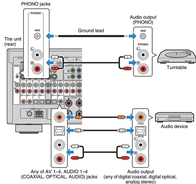
If you select the input source by pressing AV 1-4, AUDIO 1-4 or PHONO on the remote control, the audio played back on the audio device will be output from the unit.
