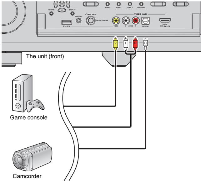
If you select “V-AUX” as the input source by pressing V-AUX, the video/audio played back on the device will be output from the unit.
